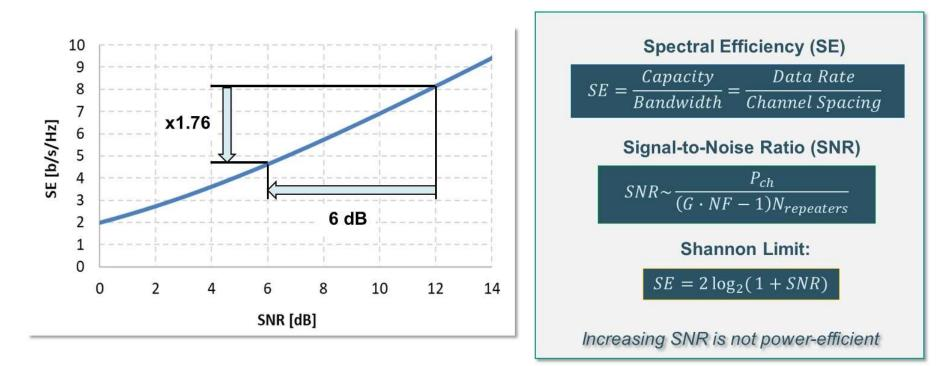
Sharing repeater power across parallel paths is a power efficient approach to increased capacity
